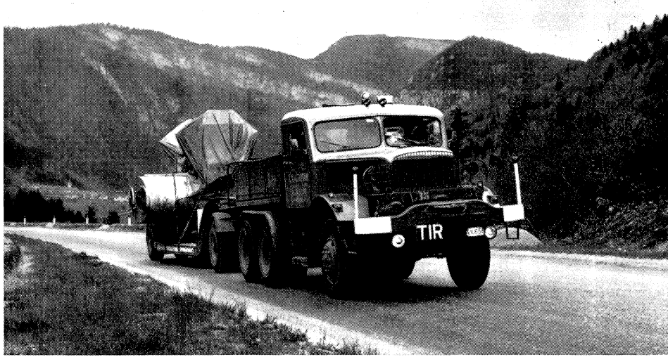
3. The complete vacuum-tank assembly, including the chamber body, expansion system, thermal shields, etc., was transported from the Rutherford Laboratory to CERN in May 1963. A low maximum speed was enforced to prevent undue vibration of the more delicate parts, and the physicist in charge kept a bicycle pump ready to ensure that the pressure in the inflatable sealing gaskets was always sufficiently high to prevent vibration of the thick glass windows of the chamber. The lorry with its 30-ton load is seen here in France, coming through the Jura mountains.
